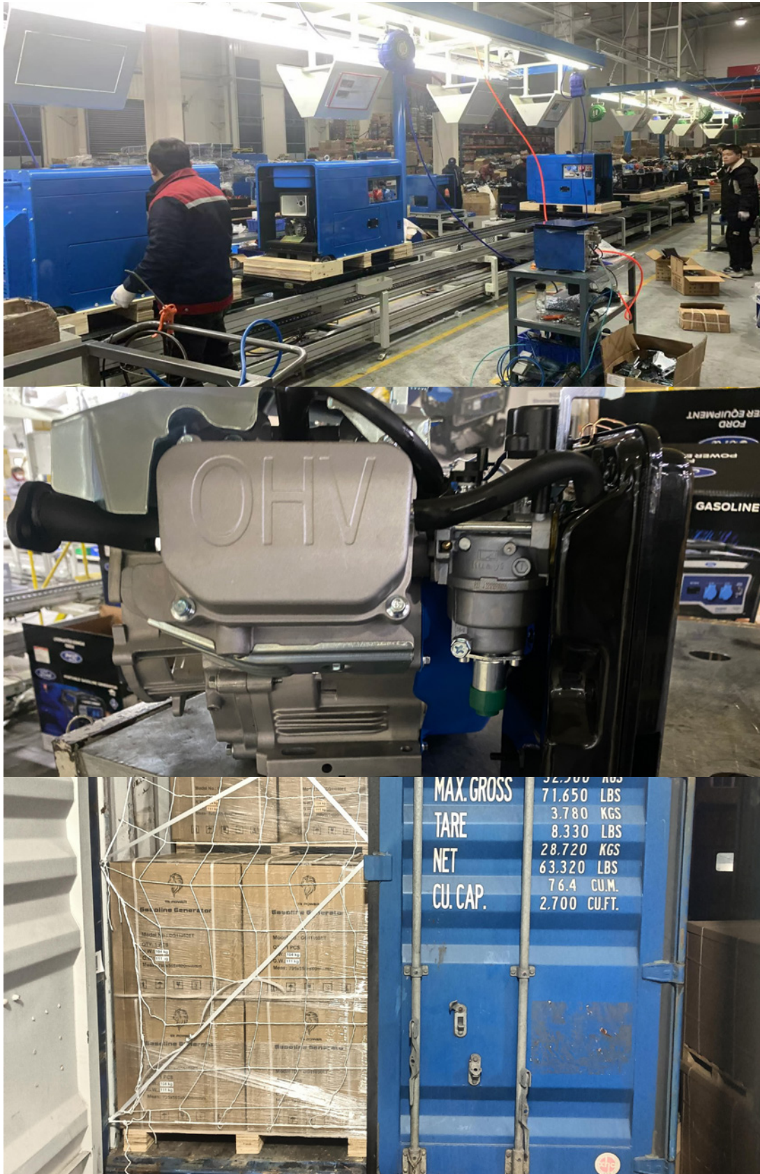
Caption: (top) assembly line for the production of the 8.2 kW diesel generators, (middle) parts assembly of an 8.5 kW generator and (bottom) one of four containers being stacked till to the door before being shipped by train to Poland.
